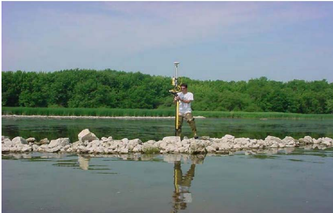
Figure 43. 6/13/03; USGS Gage - 776.31 msl; top of riprap protection at Carcajou Shallow Marsh at outside corner of riprap lakeward from opening behind Carcajou Shallow Marsh. Elevation near top of rock is 777.48 msl.
